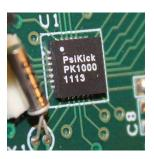
Low-power chip: PsiKick's first low-power chip runs on harvested energy. It includes only a subset of components that the company plans to incorporate on its first commercially available chip.
