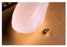
cubic millimeters, or about a tenth the size of IBM's former recordsetter. It's so small that one grain of rice seems gigantic in comparison -- and it's so sensitive that its transmission LED could instigate currents in its circuits.
