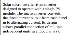
Micro-inverter advantages include single panel power optimization, independent operation of each panel, plug-and play installation, improved installation and fire safety, minimized costs with system design and stock minimization.
