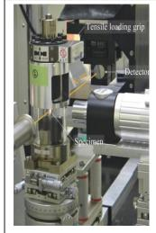
Non-destructive observation of internal fatiguecrack growth in Ti–6AI–4V by usingsynchrotro n radiation µCTimaging
