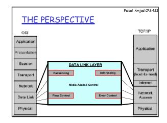
Data can be corrupted during transmission, for reliable communication errors must be detected and corrected
